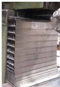
* Example of bellows with stainless steel strips recommended for areas with hot shavings.
